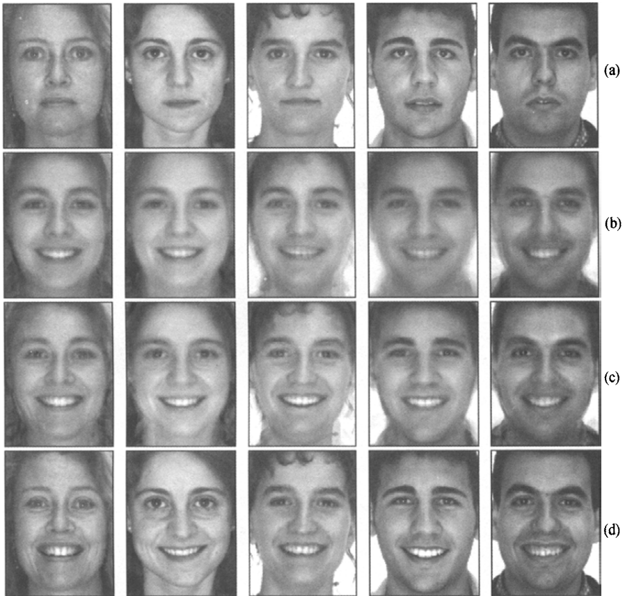
Fig. 5.7 The results of hallucinated happy facial expressions. (a) The input neutral face images; (b) The preliminary results of manifold learning and inference; (c) The final results enhanced by belief propagation and graph cuts; (d) The ground-truth face images with happy facial expression
